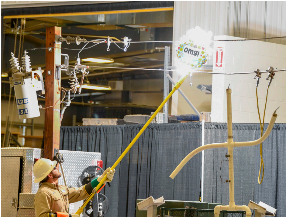
Entangled in the demonstration power line, the Mylar balloon catches fire and causes sparks on the line.
